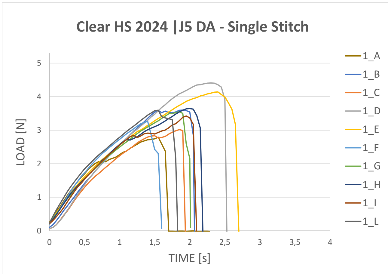
Figure 2: Results of single stitch traction tests on the 10 Elastico™ Clear High Strength Suture Preset samples.
